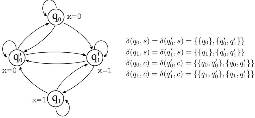
Figure 4. An ATS for the controller/client problem
